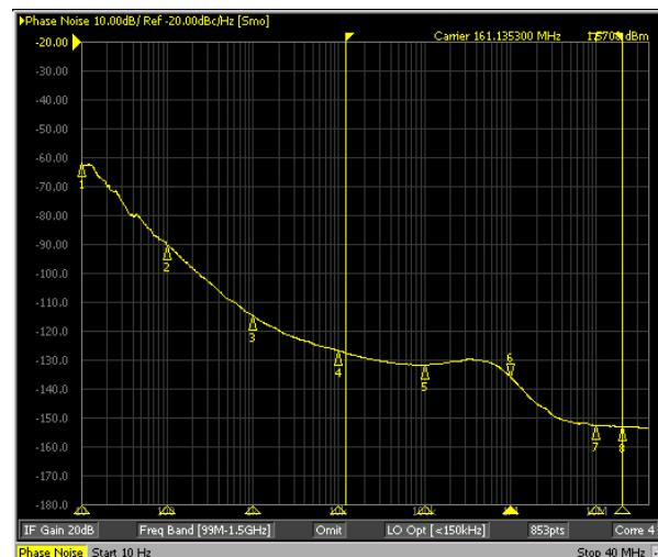
**Fractional-N Output RMS Phase Jitter = 371 fs !!**
