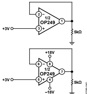
Figure 40. Burn-In Circuit
