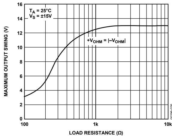
Figure 26. Maximum Output Voltage Swing vs. Load Resistance
