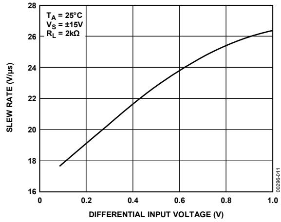
Figure 11. Slew Rate vs. Differential Input Voltage
