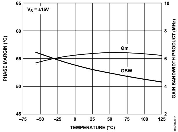
Figure 7. Phase Margin, Gain Bandwidth Product vs. Temperature
