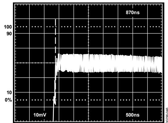
Figure 46. Settling Characteristics of the OP249 to 0.01%
