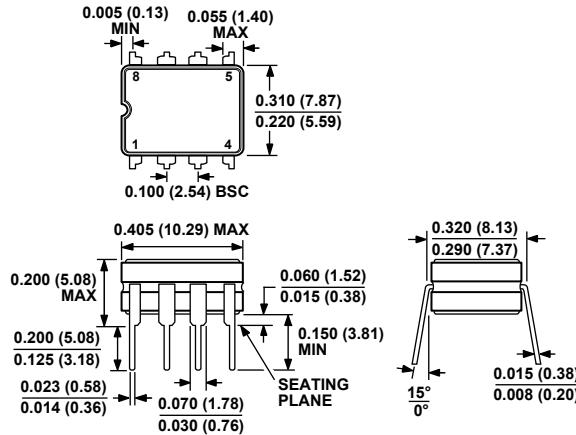
CONTROLLING DIMENSIONS ARE IN INCHES; MILLIMETER DIMENSIONS
