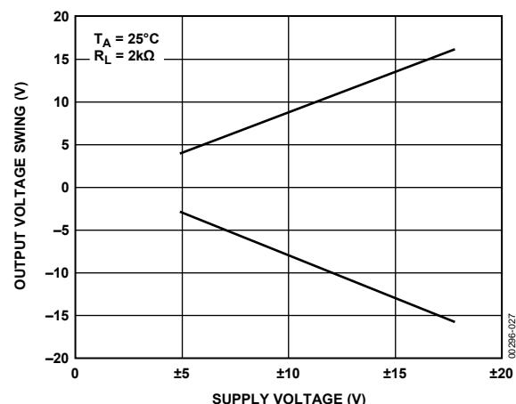
Figure 27. Output Voltage Swing vs. Supply Voltage
