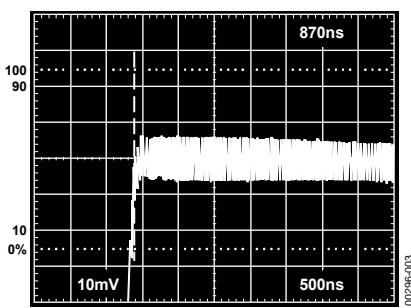
Figure 3. Fast Settling (0.01%)
