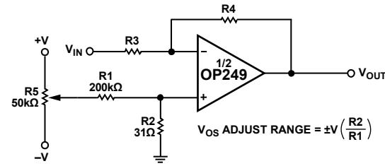
Figure 44. Offset Adjustment for Inverting Amplifier Configuration
