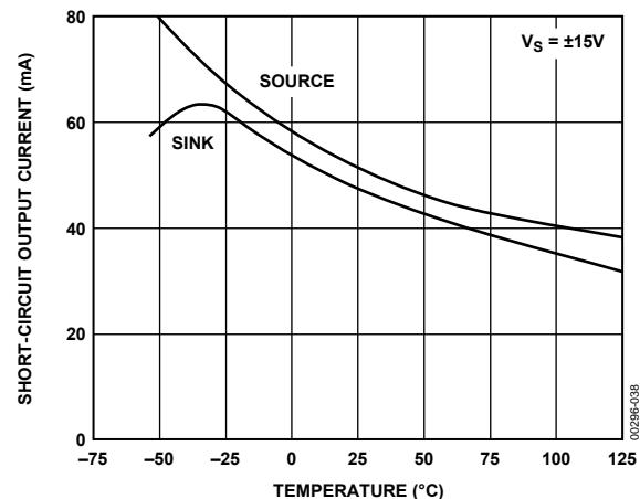
Figure 38. Short-Circuit Output Current vs. Junction Temperature
