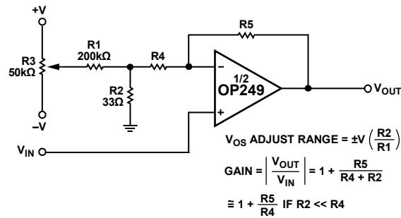
Figure 45. Offset Adjustment for Noninverting Amplifier Configuration
