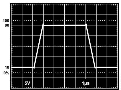
Figure 5. Excellent Output Drive,  $R_L = 600\text{ }\Omega$
