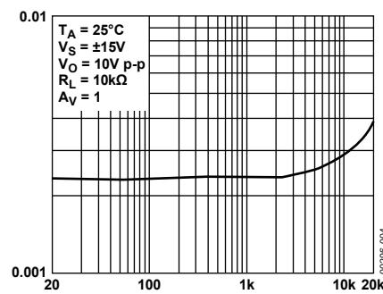
Figure 4. Low Distortion,  $A_V = 1$ ,  $R_L = 10\text{ k}\Omega$
