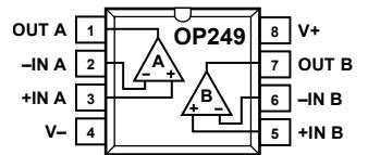
Figure 1. 8-Lead CERDIP (Q-8) and
