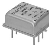
The MS18-1006 is an optically coupled SSR employing power MOSFET output chips in an inverse series configuration for switching DC or bi-directional loads. A common source connection is provided for the user to
