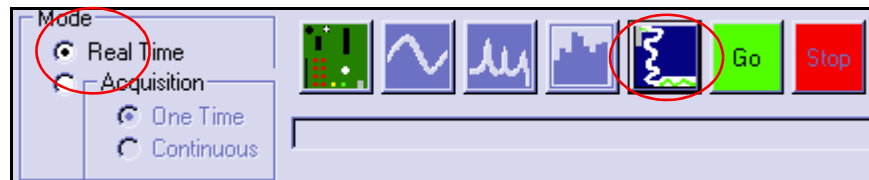
FIGURE 2-6: Selecting the Strip Chart Tool for Real-time Temperature Display.
