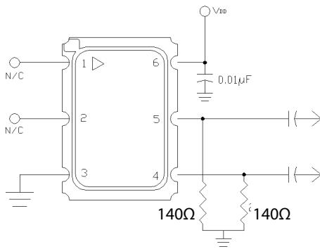
**Figure 7. Single Resistor Termination Scheme**
