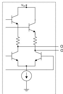
**Figure 9. Standard LVDS Output Configuration**
