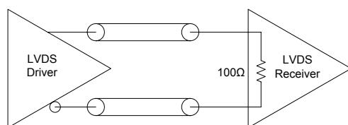
**Figure 10. LVDS to LVDS Connection, Internal 100ohm**
