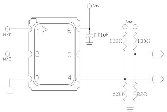
**Figure 8. Pull-Up Pull Down Termination**
