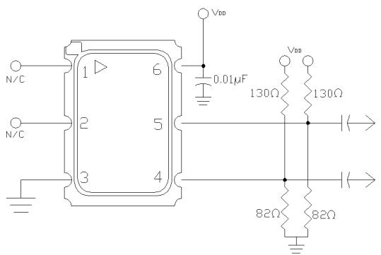
**Figure 8. Pull-Up Pull Down Termination**
