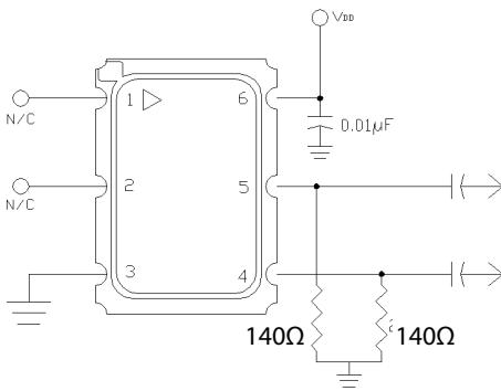
**Figure 7. Single Resistor Termination Scheme**
