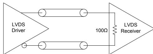
**Figure 10. LVDS to LVDS Connection, Internal 100ohm**
