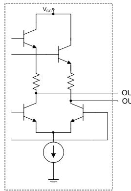
**Figure 9. Standard LVDS Output Configuration**
