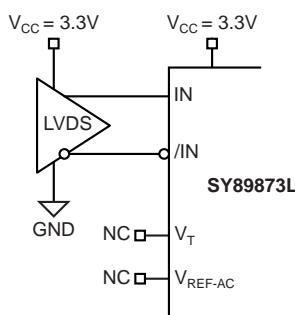
**Figure 3e. LVDS Input Interface****Figure 3f. HSTL Input Interface****RELATED MICREL PRODUCTS AND SUPPORT DOCUMENTATION**
