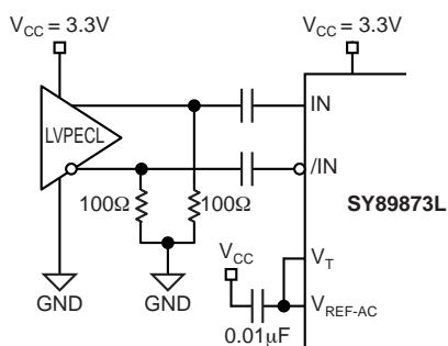
**Figure 3d. AC-Coupled LVPECL Input Interface**
