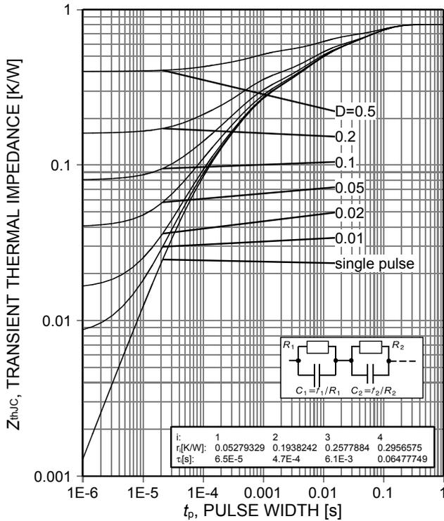
Figure 21. IGBT transient thermal impedance ( $D=t_p/T$ )
