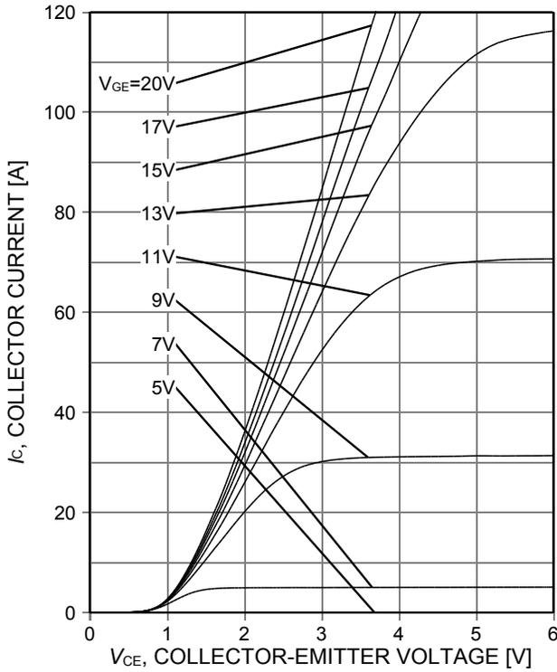
Figure 5. Typical output characteristic ( $T_j=25^\circ\text{C}$ )
