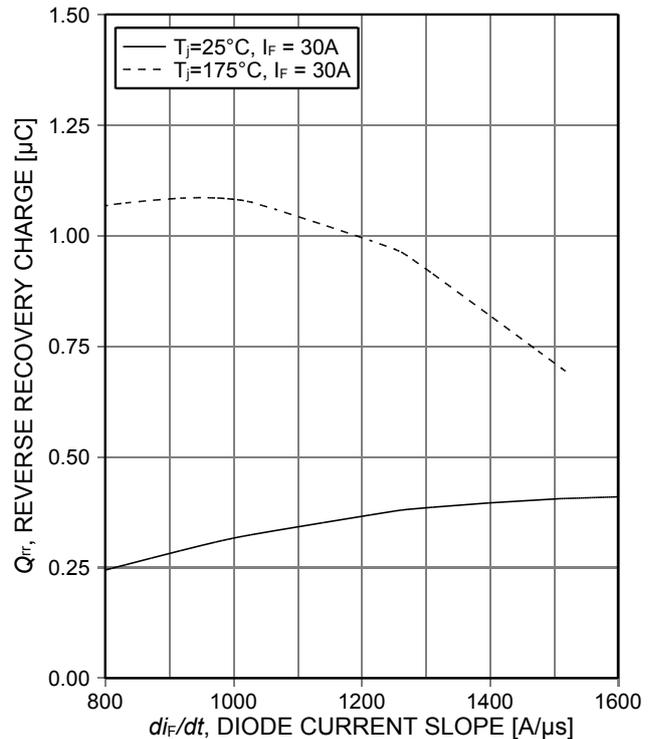
Figure 24. Typical reverse recovery charge as a function of diode current slope ( $V_R=400V$ )
