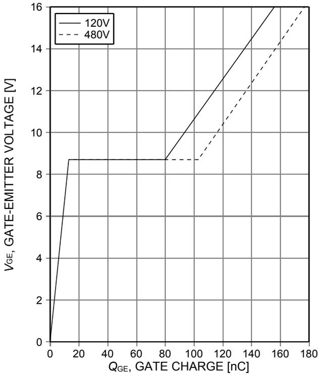
Figure 17. **Typical gate charge**
