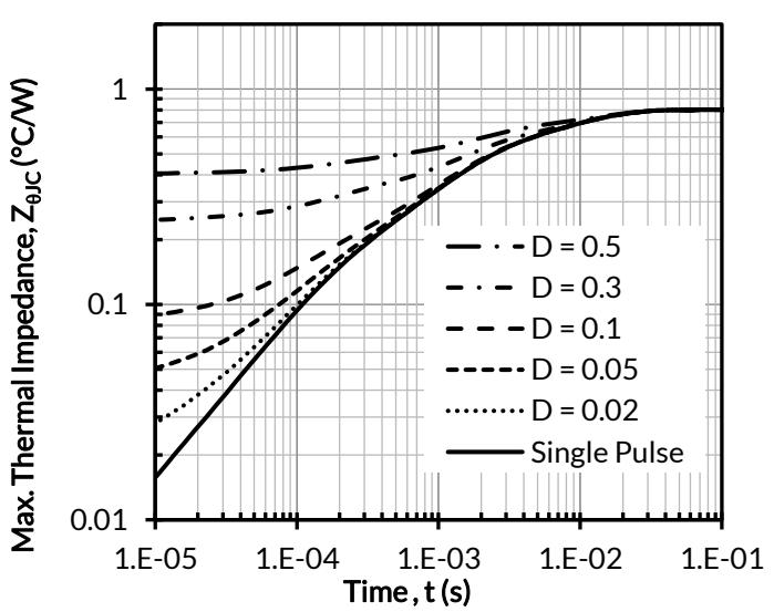
Figure 6. Maximum transient thermal impedance
