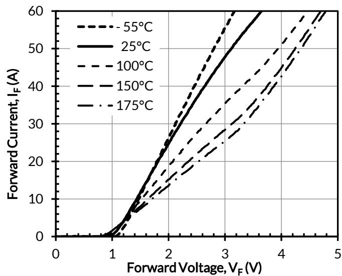
Figure 2. Typical forward characteristics in surge current
