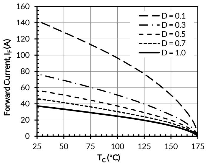
Figure 5. Diode forward current
