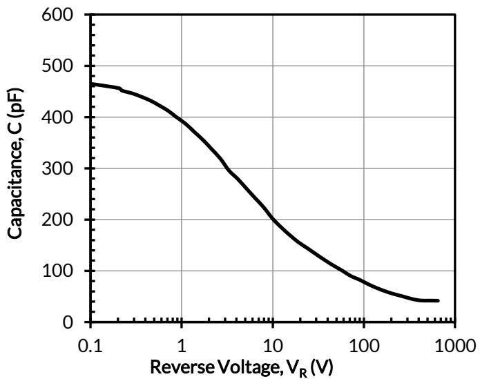
Figure 7. Capacitance vs. reverse voltage at 1MHz
