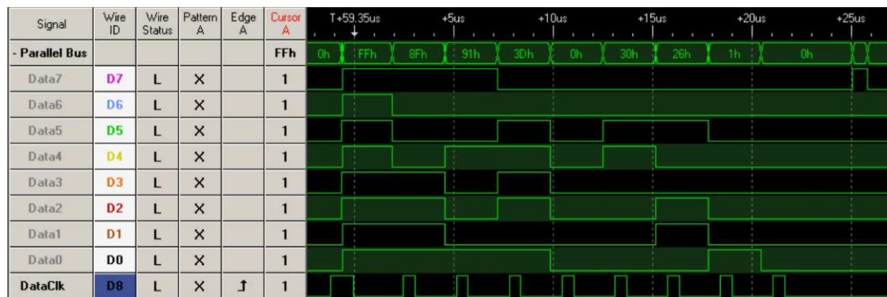
Figure 5-13. Parallel Interface Communication With Continuous Stop Condition
