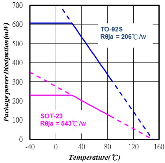
Figure 8. Temperature vs. Power Dissipation
