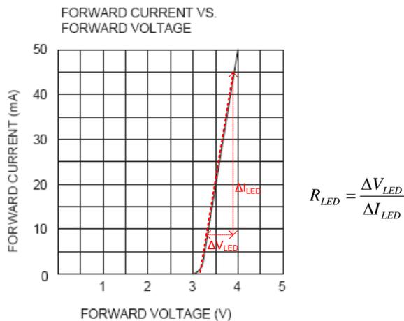
Figure 5: LED Dynamic Resistance Equivalent
