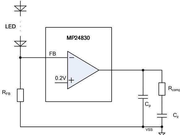
Figure 4: RCC Compensation Network on COMP Pin
