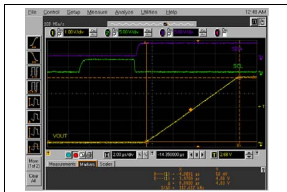
FIGURE 2-96: Full-Scale Settling Time (000h to FFFh) (MCP4726).
