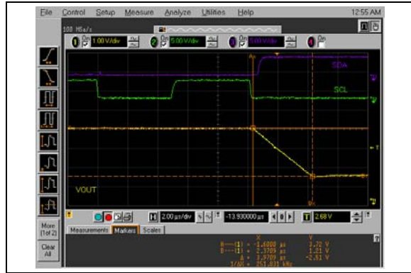
FIGURE 2-99: Half-Scale Settling Time (C00h to 400h) (MCP4726).
