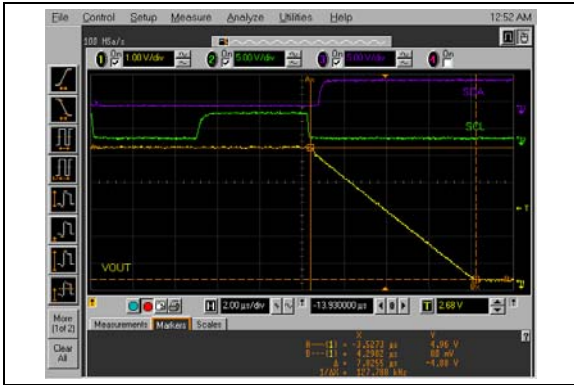
FIGURE 2-97: Full-Scale Settling Time (FFFh to 000h) (MCP4726).
