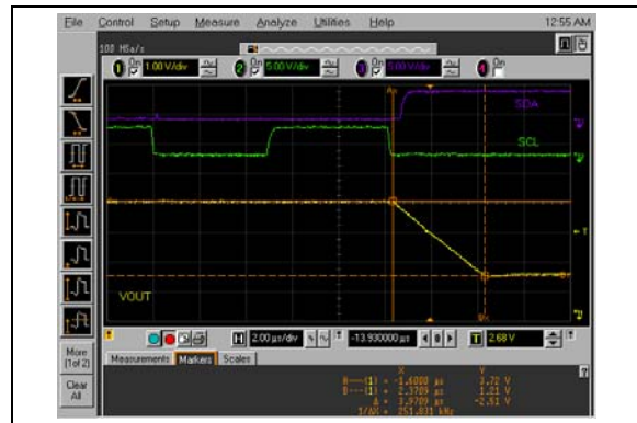
FIGURE 2-99: Half-Scale Settling Time (C00h to 400h) (MCP4726).
