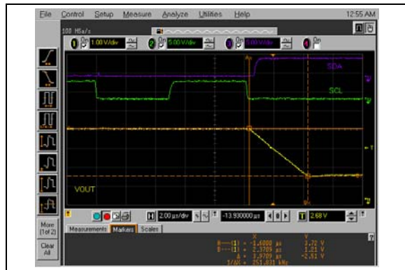
FIGURE 2-99: Half-Scale Settling Time (C00h to 400h) (MCP4726).
