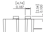
C- Two Ports Cut 0.100" Configuration
