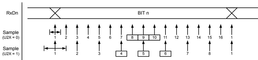
The decision of the logic level of the received bit is taken by doing a majority voting of the logic value to the three samples in the center of the received bit: If two or all three center samples (those marked by
