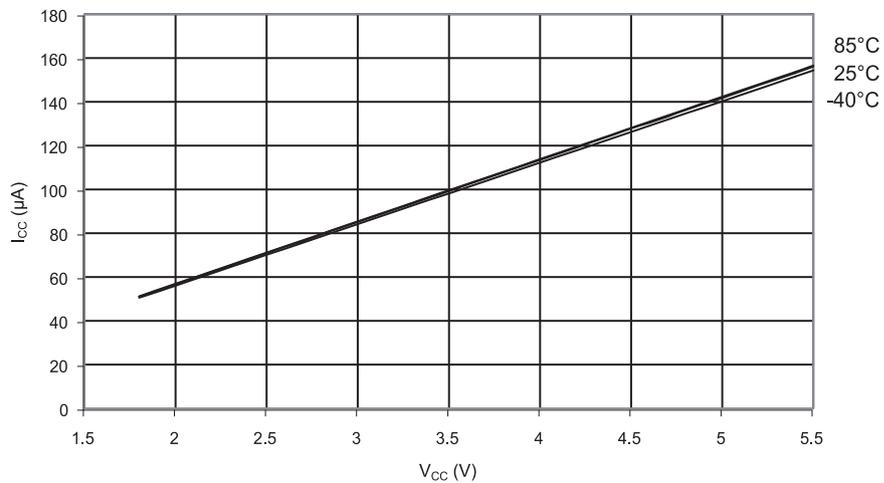
**Figure 34-47. Brownout Detector Current vs. V<sub>CC</sub>**
