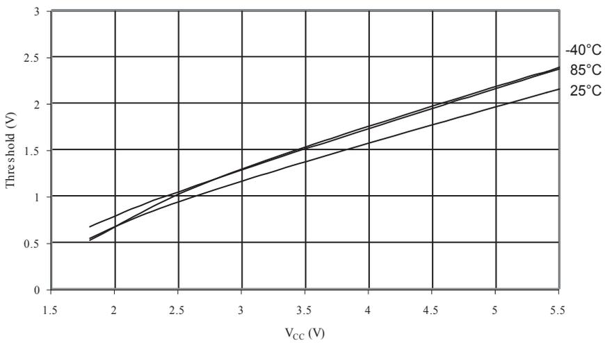
Figure 34-33. Reset Pin Input Hysteresis vs.  $V_{CC}$
