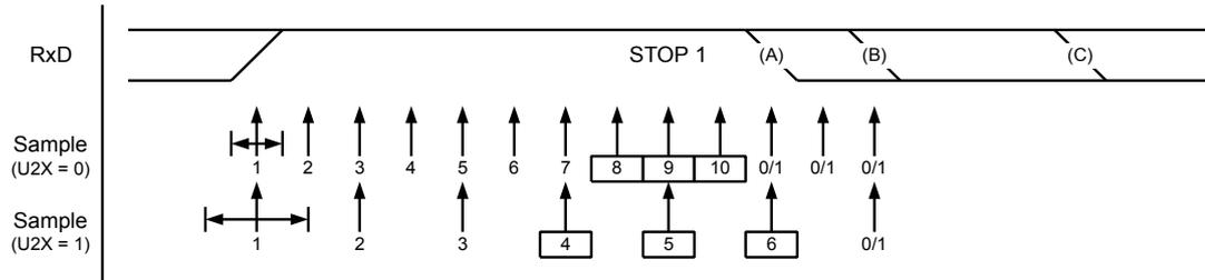
The same majority voting is done to the stop bit as done for the other bits in the frame. If the stop bit is registered to have a logic '0' value, the Frame Error (UCSRnA.FE) Flag will be set.
