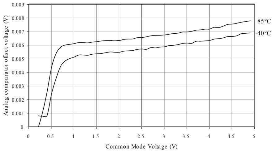
**Figure 34-43. Analog comparator offset voltage vs. common mode voltage (V<sub>CC</sub> = 2.7V).**
