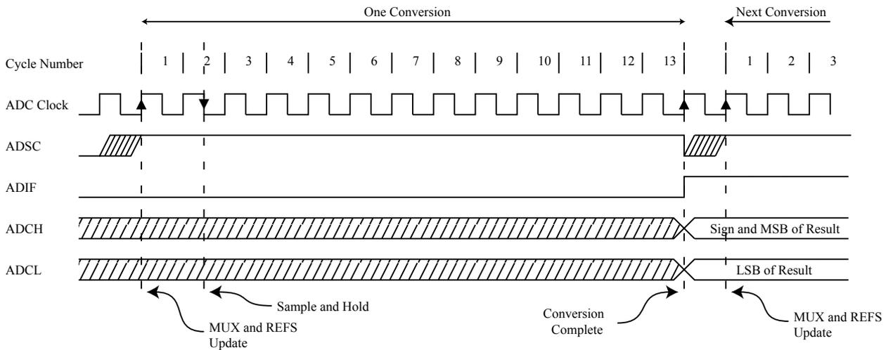
**Figure 28-6. ADC Timing Diagram, Auto Triggered Conversion**
