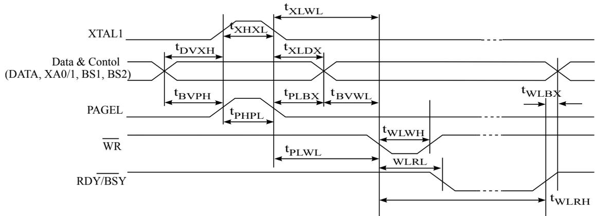
**Figure 33-8. Parallel Programming Timing, Loading Sequence with Timing Requirements**
