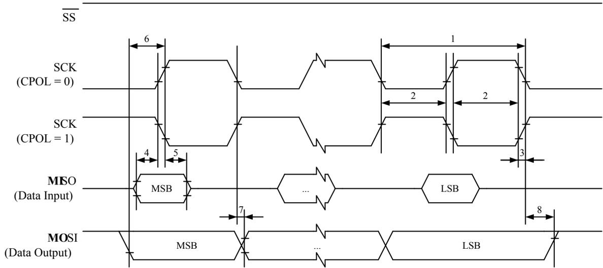
**Figure 33-5. SPI Interface Timing Requirements (Slave Mode)**
