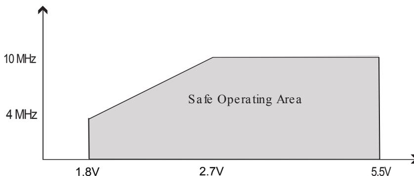
**Figure 33-2. Maximum Frequency vs.  $V_{CC}$  for ATmega48/88/168**
