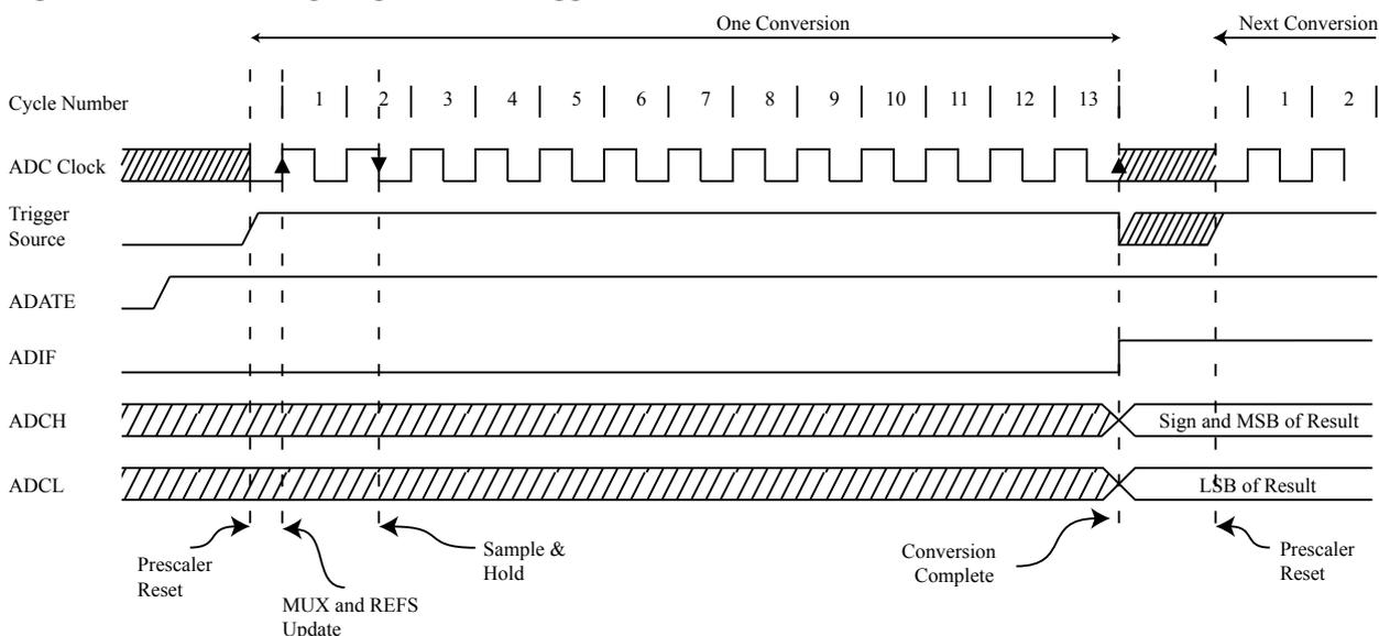
**Figure 28-7. ADC Timing Diagram, Free Running Conversion**
