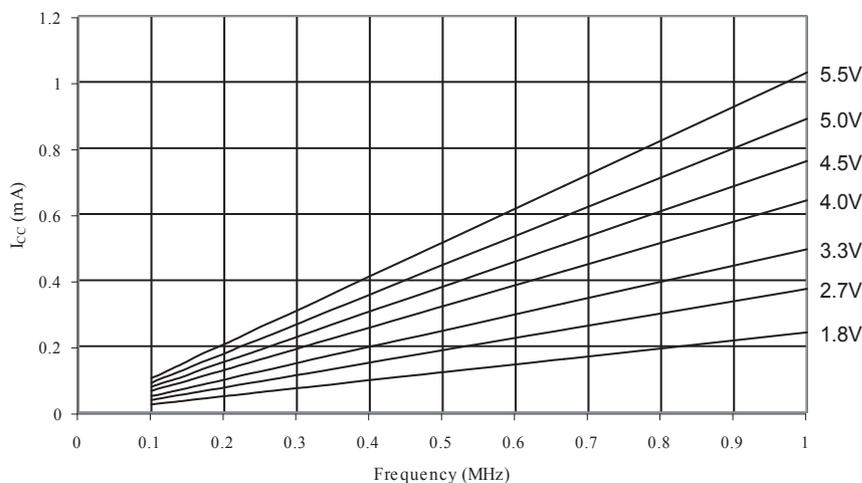
**Figure 34-2. Active Supply Current vs. Frequency (1MHz - 24MHz)**
