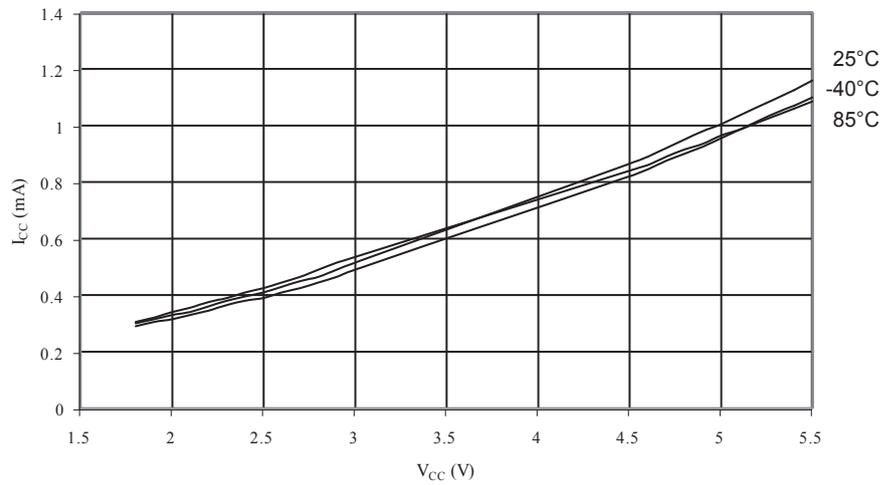
Figure 34-5. Active Supply Current vs.  $V_{CC}$  (Internal RC Oscillator, 8MHz)
