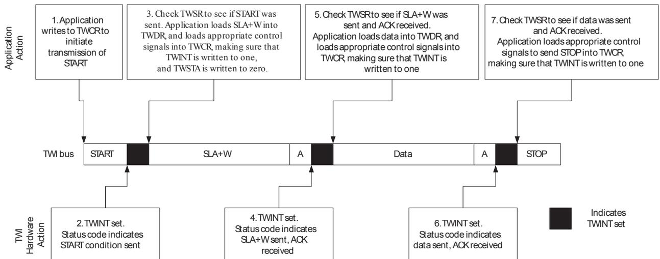
1. The first step in a TWI transmission is to transmit a START condition. This is done by writing a specific value into TWCRn, instructing the TWI n hardware to transmit a START condition. Which value to write is described later on. However, it is important that the TWINT bit is set in the value written. Writing a one to TWINT clears the flag. The TWI n will not start any operation as long as the
