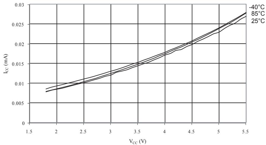
**Figure 34-10. Idle Supply Current vs.  $V_{CC}$  (Internal RC Oscillator, 1MHz)**
