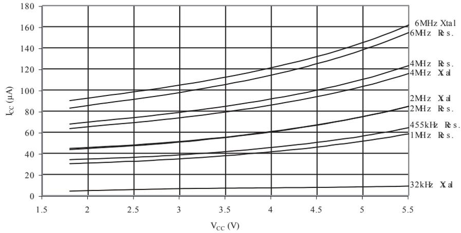
**Figure 34-17. Standby supply current vs.  $V_{CC}$  (full swing crystal oscillator)**
