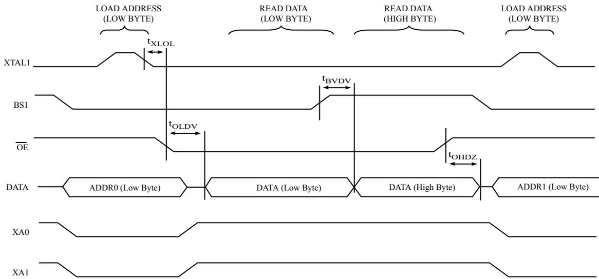
**Note:** The timing requirements shown in [Table 33-11](#) (i.e.,  $t_{DVXH}$ ,  $t_{XHXL}$ , and  $t_{XLDX}$ ) also apply to reading operation.
