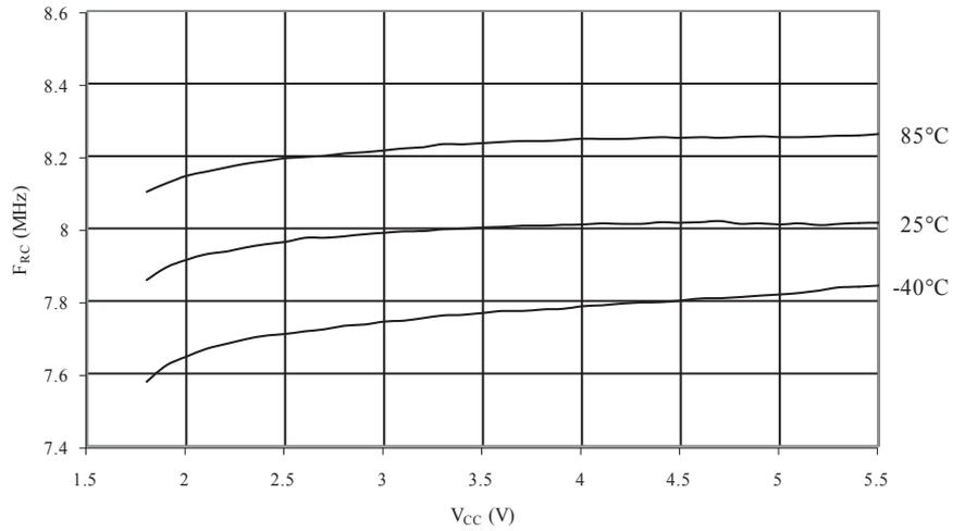
**Figure 34-36. Calibrated 8MHz RC Oscillator Frequency vs. Temperature**
