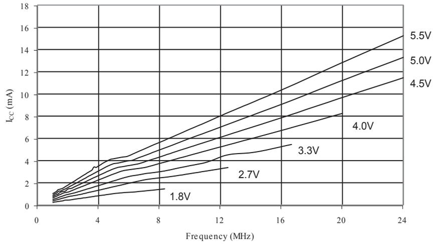
**Figure 34-3. Active Supply Current vs.  $V_{CC}$  (Internal RC Oscillator, 128kHz)**
