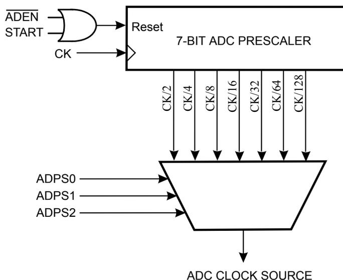
By default, the successive approximation circuitry requires an input clock frequency between 50kHz and 200kHz to get maximum resolution. If a lower resolution than 10 bits is needed, the input clock frequency to the ADC can be higher than 200kHz to get a higher sample rate.
