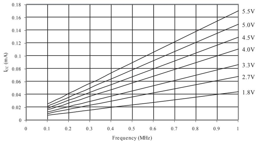
**Figure 34-50. Reset Supply Current vs. Frequency (1MHz - 24MHz)**
