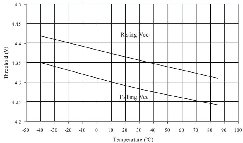
**Figure 34-41. Bandgap voltage vs. VCC**
