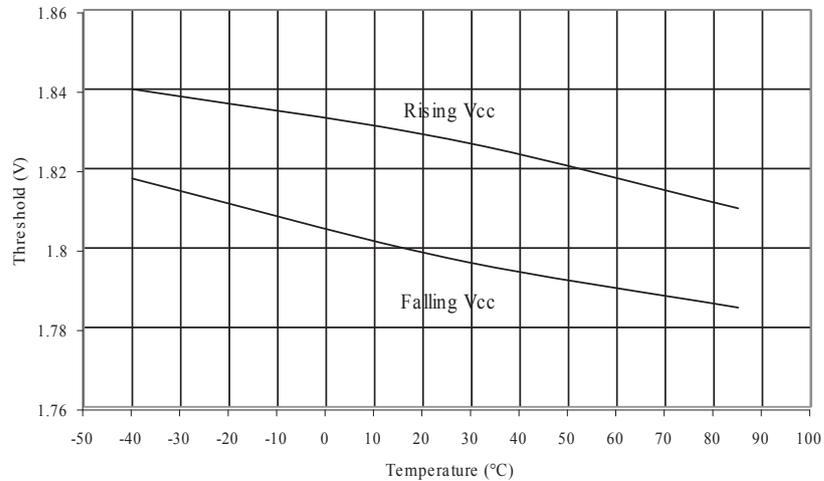
Figure 34-39. BOD Thresholds vs. Temperature (BODLEVEL is 2.7V)
