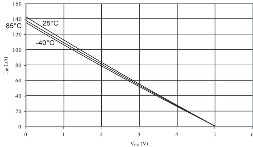
**Figure 34-20. Reset Pull-up Resistor Current vs. Reset Pin Voltage ( $V_{CC} = 2.7V$ )**
