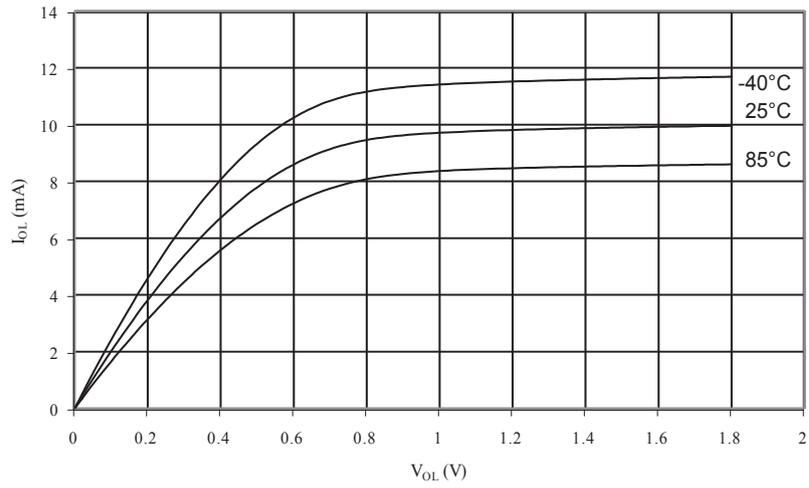
**Figure 34-25. I/O Pin Output Voltage vs. Source Current ( $V_{CC} = 5V$ )**
