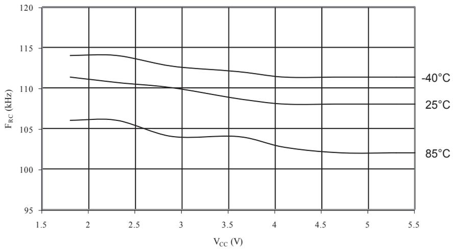
**Figure 34-35. Calibrated 8 MHz RC Oscillator Frequency vs.  $V_{CC}$**
