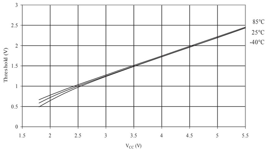
**Figure 34-30. I/O Pin Input Hysteresis vs.  $V_{CC}$**
