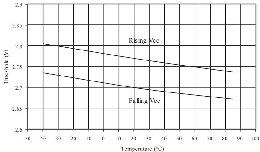
Figure 34-40. BOD Thresholds vs. Temperature (BODLEVEL is 4.3V)
