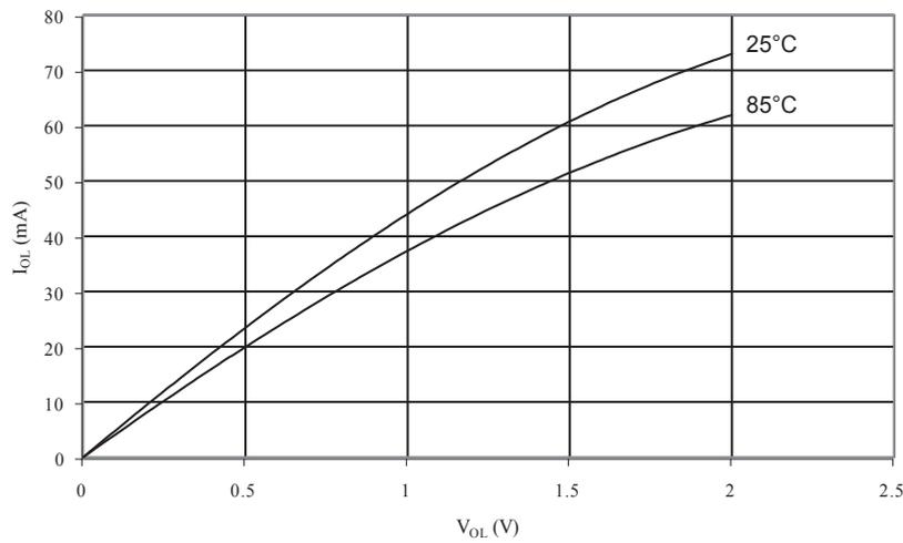
Figure 34-23. I/O Pin Output Voltage vs. Sink Current ( $V_{CC} = 2.7V$ )
