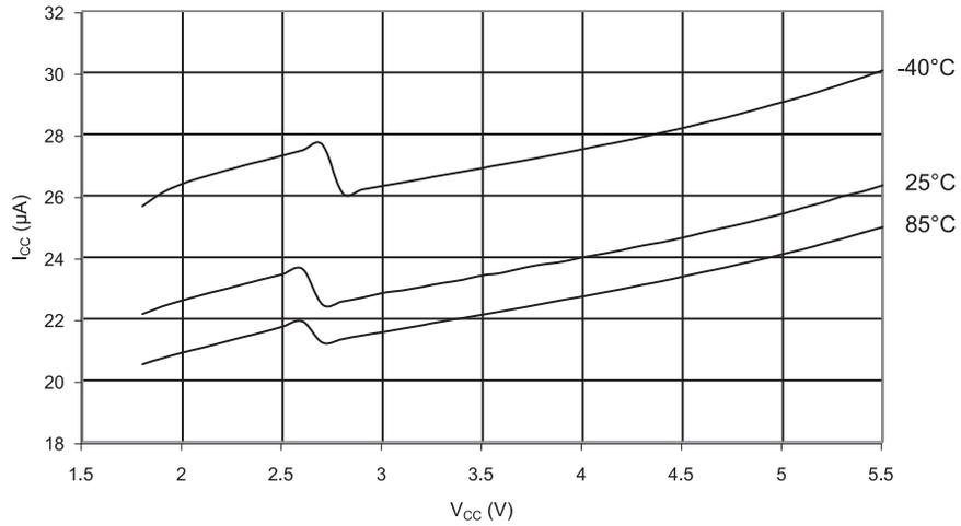
**Figure 34-48. Programming Current vs. V<sub>CC</sub>**
