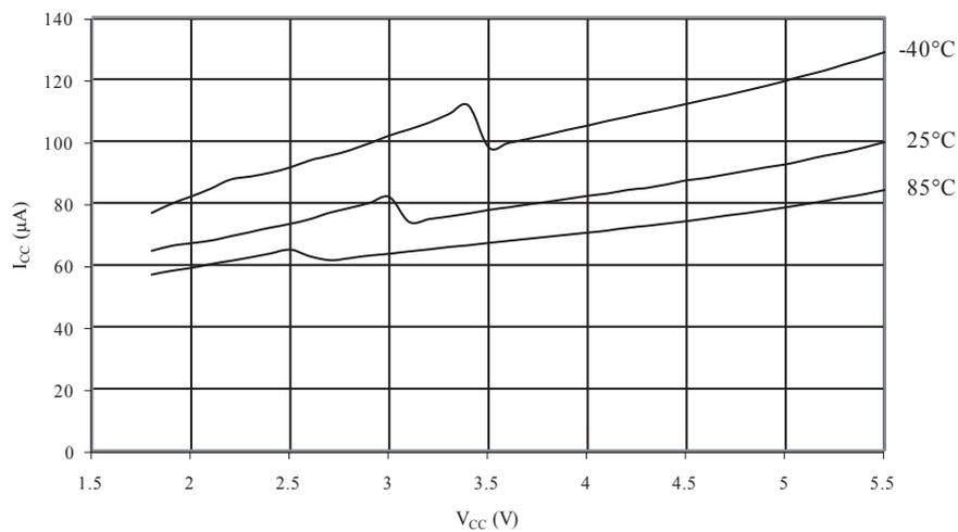
Figure 34-46. AREF External Reference Current vs.  $V_{CC}$
