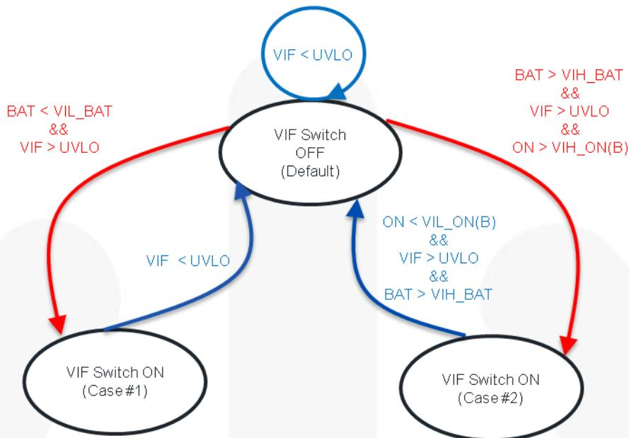
Figure 11. V<sub>IF</sub> Turn-On Qualification State Diagram
