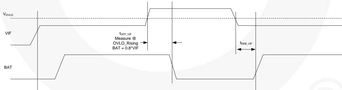
Figure 10. Timing for  $V_{IF}$  OVLO Operation (ON=Don't Care)
