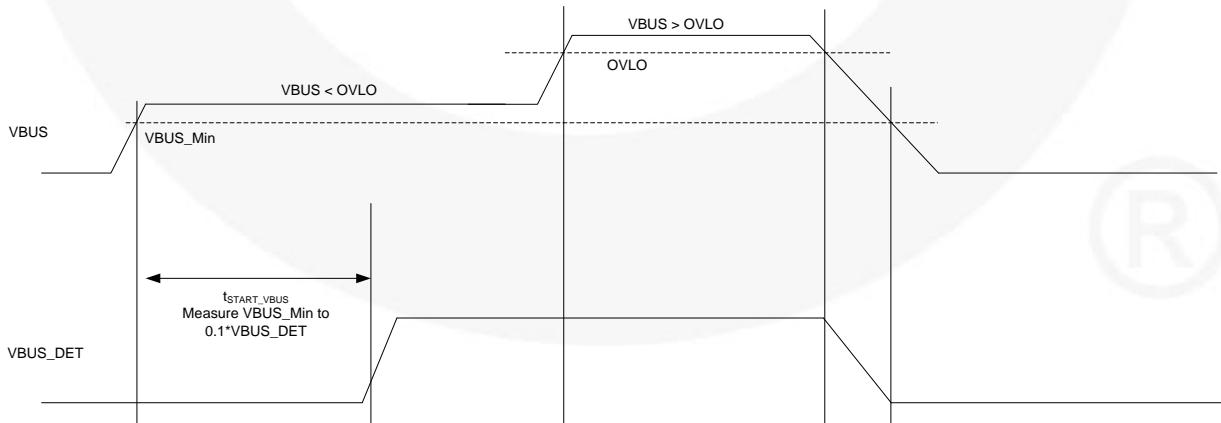
Figure 7. Always ON V<sub>BUS\_DET</sub> Operation (ONB=HIGH)
