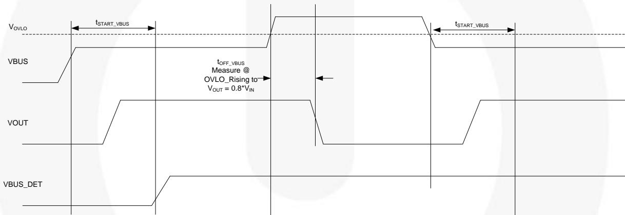
Figure 6. Timing for V<sub>BUS</sub> OVLO Operation (ONB=LOW)
