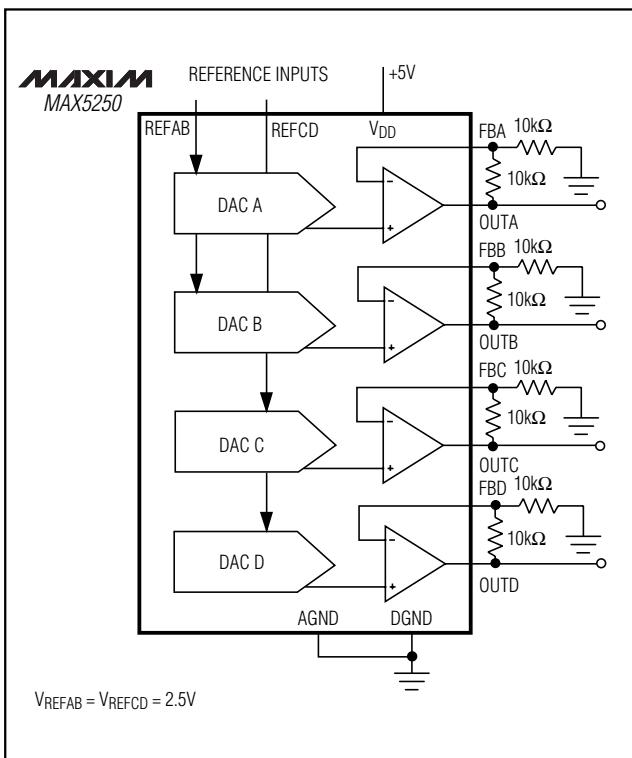
Figure 10. Unipolar Rail-to-Rail Output Circuit
