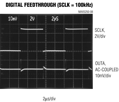
$\overline{CS} = \overline{PDL} = \overline{CL} = 5V$ ,  $DIN = 0V$
