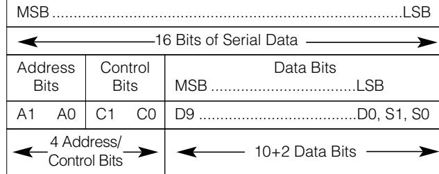
Figure 4. Serial-Data Format
