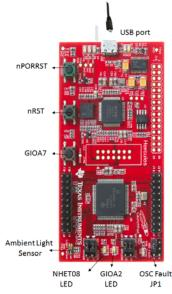
Upon detecting the fault, on-board Hercules MCU will respond by asserting the error pin (nERROR) low, indicated by the red LED on the bottom right corner of the board. **Note**: Open jumper JP1 and reset the board before continuing with other demos.
