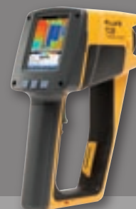
Fluke Ti20 Thermal Imager
