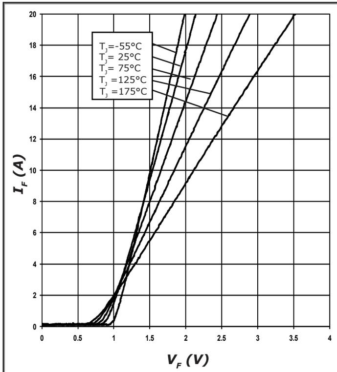
Figure 1. Forward Characteristics
