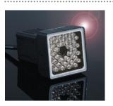
The Built-in lighting camera and improved controller brings about an even higher degree of automatic lighting. With this camera you can produce up to a maximum of 1296 patterns of reflective lighting making the chore of choosing lighting equipment unnecessary. The lighting setup can be managed as digital data so it is possible to store the optimal setup for each job, and it smoothly handles the changing of settings. It is also possible to fine-tune the customized setup can be added.
