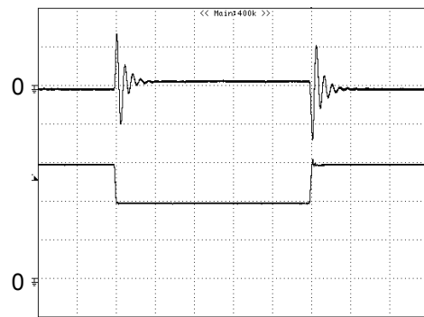
Figure 9: Output voltage response to step-change in load current (75%-50%-75% of I_o , max; di/dt = 1.0A/\mu s ). Load cap: 220 \mu F tantalum capacitor and 1 \mu F ceramic capacitor. Top Trace: V_{out} (100mV/div, 200us/div), Bottom Trace: I_{out} (10A/div). Scope measurement should be made using a BNC cable (length shorter than 20 inches). Position the load between 51 mm to 76 mm (2 inches to 3 inches) from the module
