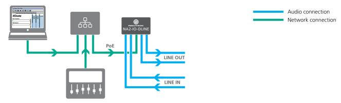
The Dante<sup>™</sup> adapter forwards information to the PoE switch indicating that it is a "Class 1" device to ensure the correct power supply.
