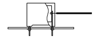
Temperature monitored inside the capacitor.
