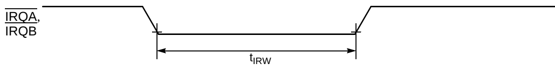
Figure 10-6 External Interrupt Timing (Negative Edge-Sensitive)
