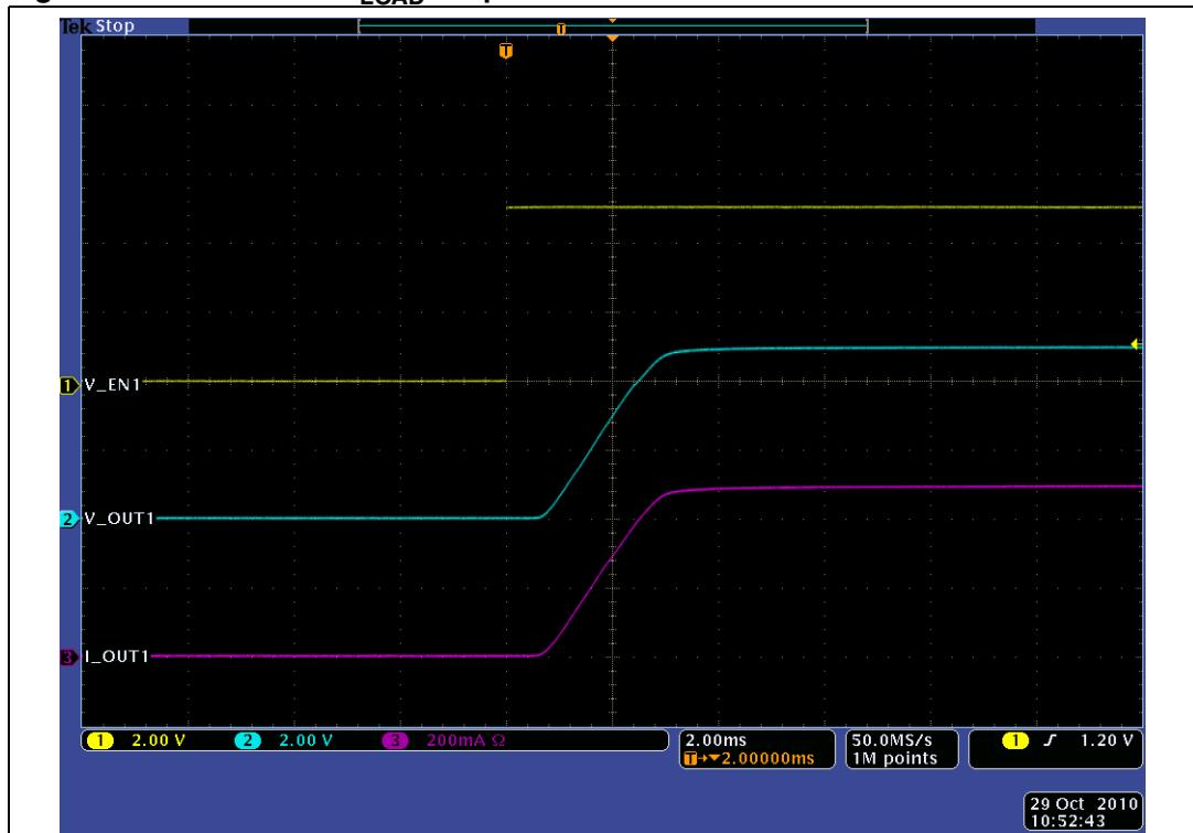
Figure 9. Turn-on for C_{LOAD} = 1 \mu F
