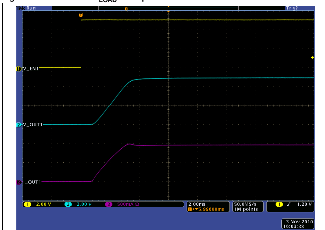
Figure 31. Turn-on for C_{LOAD} = 470\ \mu\text{F}
