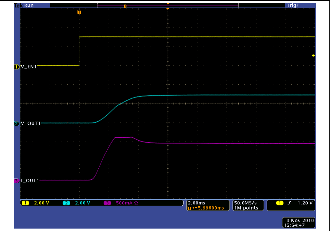
Figure 25. Turn-on for C_{LOAD} = 470\ \mu F
