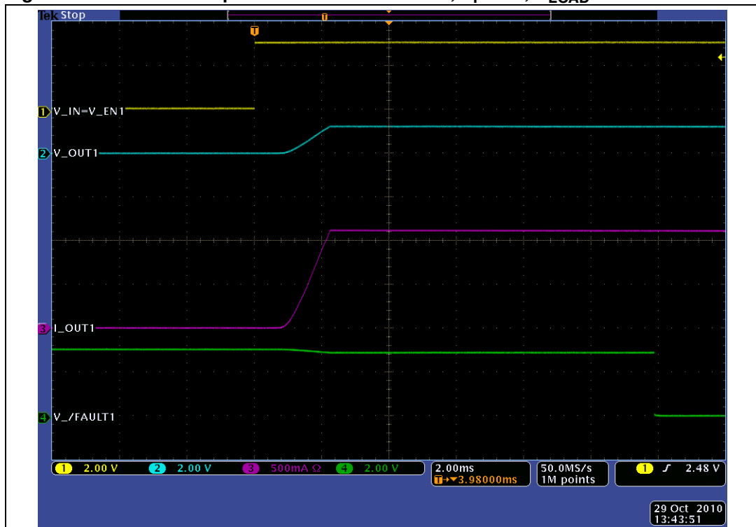
Figure 37. Overcurrent protection characteristics, V_I = 3\text{ V} , R_{LOAD} = 1\ \Omega
