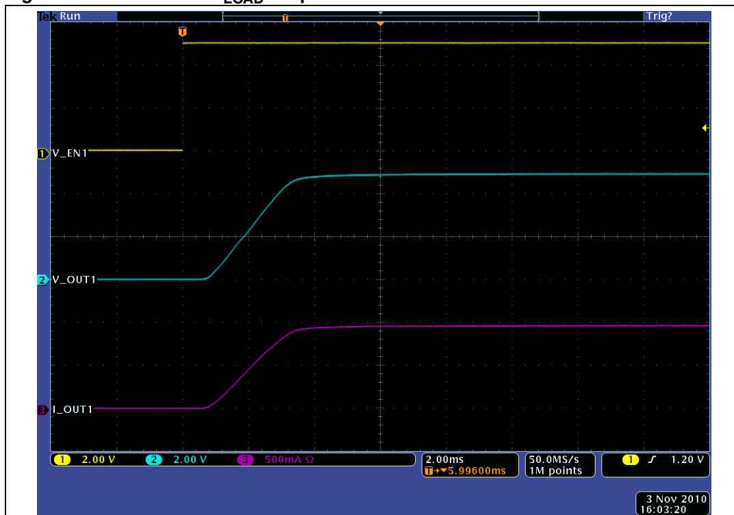
Figure 29. Turn-on for C_{LOAD} = 1 \mu F
