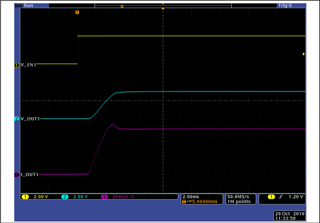
Figure 4. Turn-on for C_{LOAD} = 100\ \mu\text{F}
