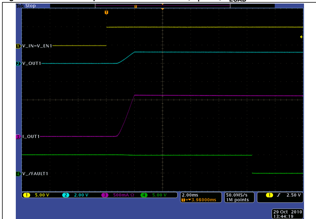
Figure 38. Overcurrent protection characteristics, V_I = 5\text{ V} , R_{LOAD} = 1\ \Omega
