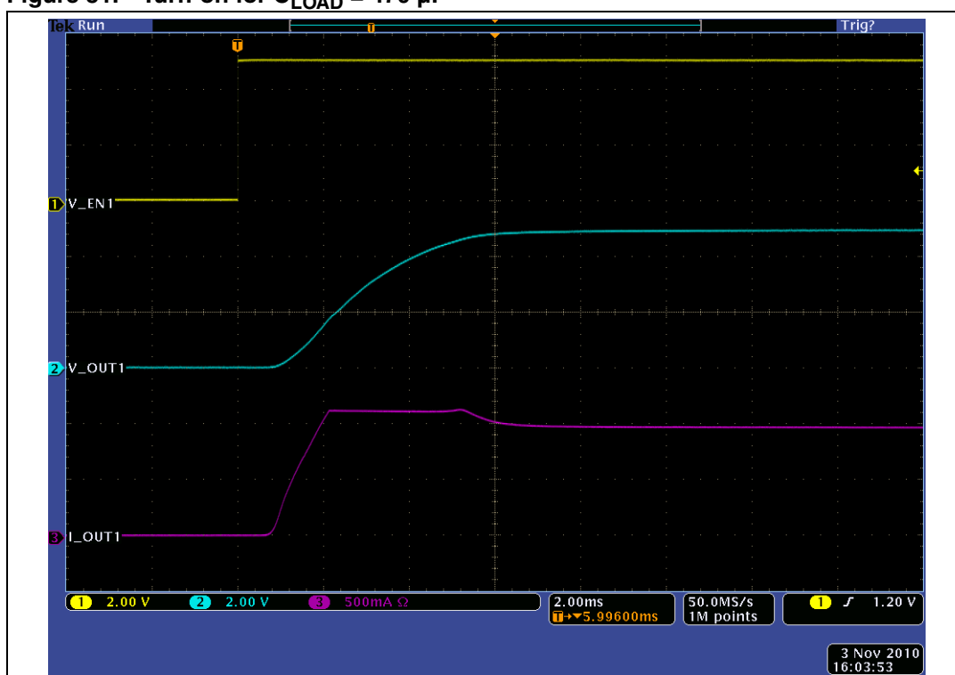
Figure 31. Turn-on for C_{LOAD} = 470\ \mu\text{F}
