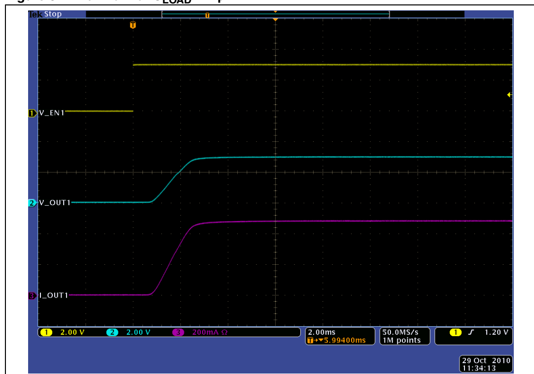
Figure 3. Turn-on for C_{LOAD} = 1\ \mu\text{F}
