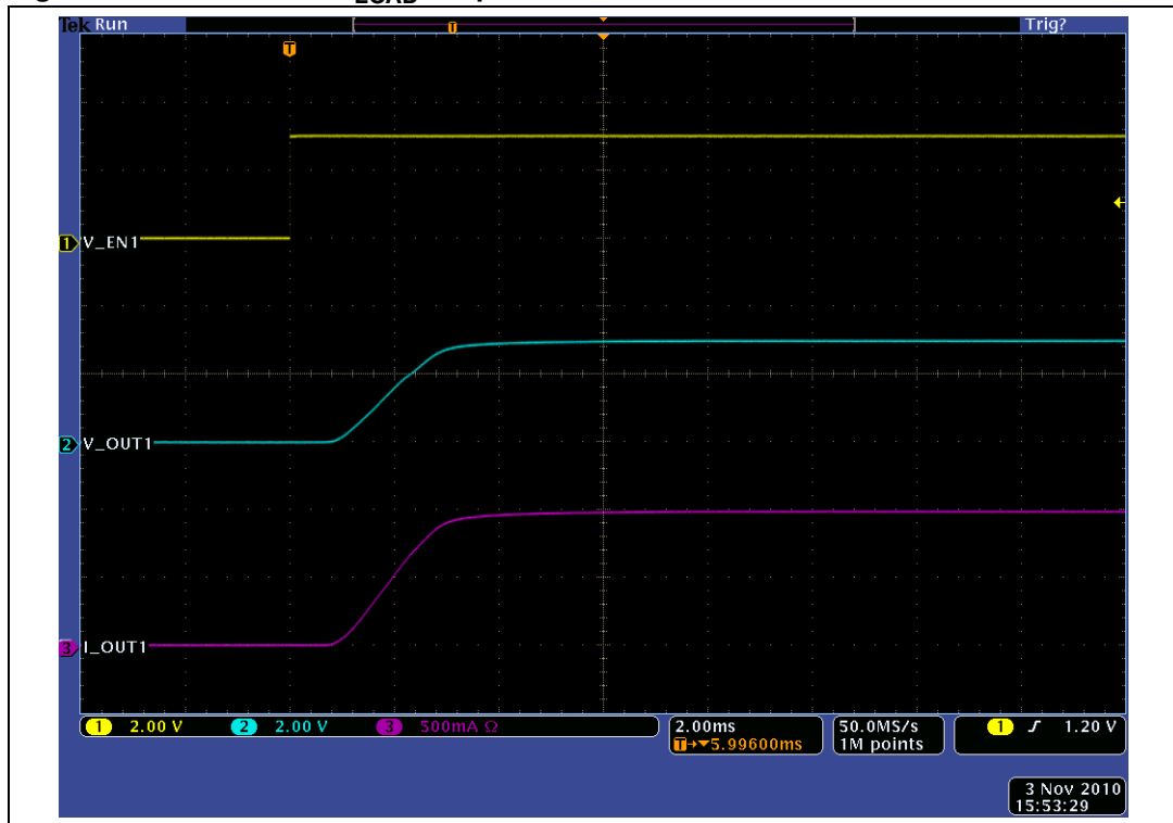
Figure 23. Turn-on for C_{LOAD} = 1\ \mu\text{F}
