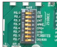
Figure 6-3: Switch 8 on the DIP switch SW15 is in ON position, DS1820 is connected to the P2.7 pin
