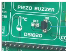
Figure 6-2: Temperature sensor DS1820 is connected
