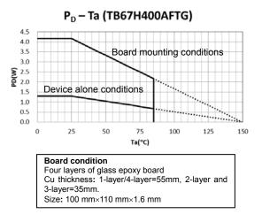
This value is dependent on a substrate pattern and mounting conditions. Moreover, when ambient temperature is high, permissible power consumption becomes small.
