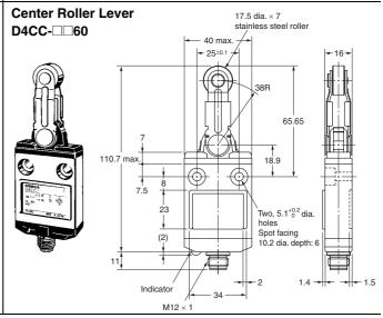
Note: Unless otherwise specified, a tolerance of  $\pm 0.4 \ \text{mm}$  applies to all dimensions.
