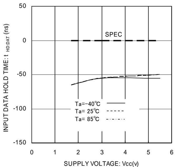
Figure 19. Input Data Hold Time t<sub>HD:DAT(HIGH)</sub>
