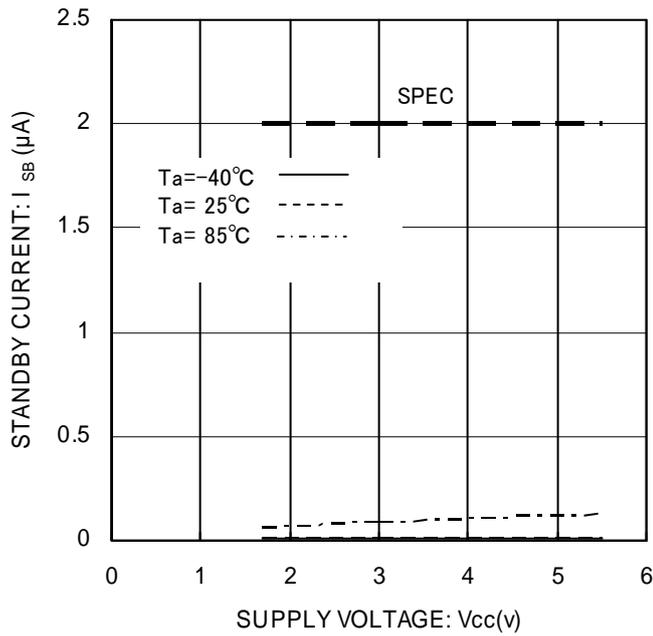
Figure 12. Standby Current I<sub>SB</sub>
