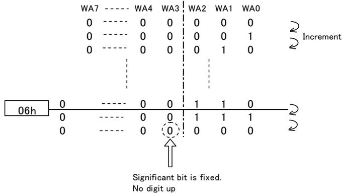
For example, when it is started from address 06h, therefore, increment is made as below, 06h→07h→00h→01h... which please note.
