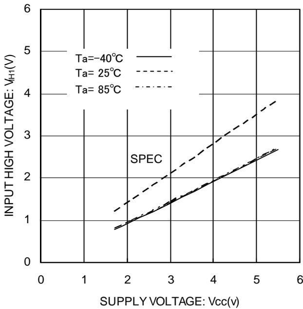
Figure 4. Input High Voltage<sub>1,2</sub>  $V_{IH1,2}$  (A0, A1, A2, SCL, SDA, WP)
