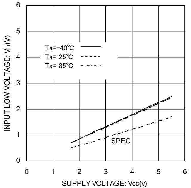
Figure 5. Input Low Voltage<sub>1,2</sub>  $V_{IL1,2}$  (A0, A1, A2, SCL, SDA, WP)
