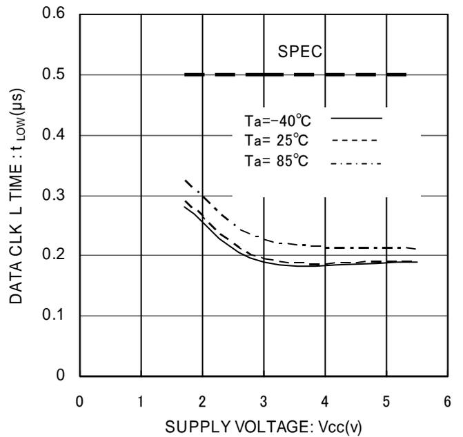
Figure 15. Data Clock Low Period t<sub>LOW</sub>
