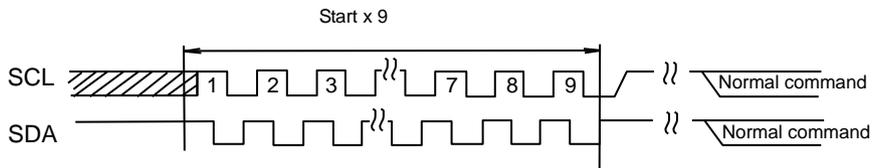
Figure 41-(c). START x 9 + command input
