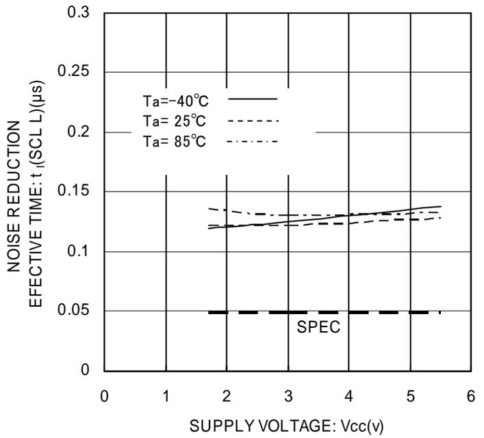
Figure 29. Noise Spike Width  $t_l$  (SCL L)
