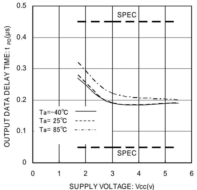
Figure 23. 'L' Output Data Delay Time tPD0
