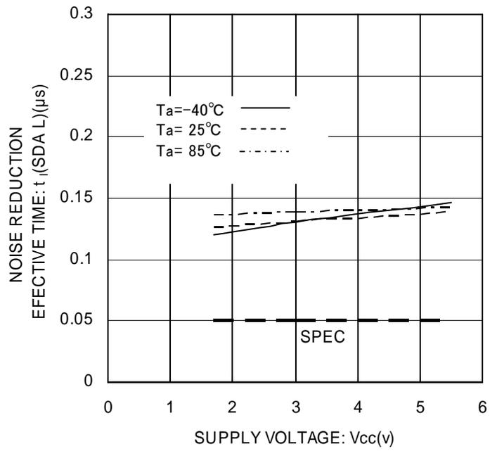
Figure 31. Noise Spike Width  $t_l$  (SDA L)
