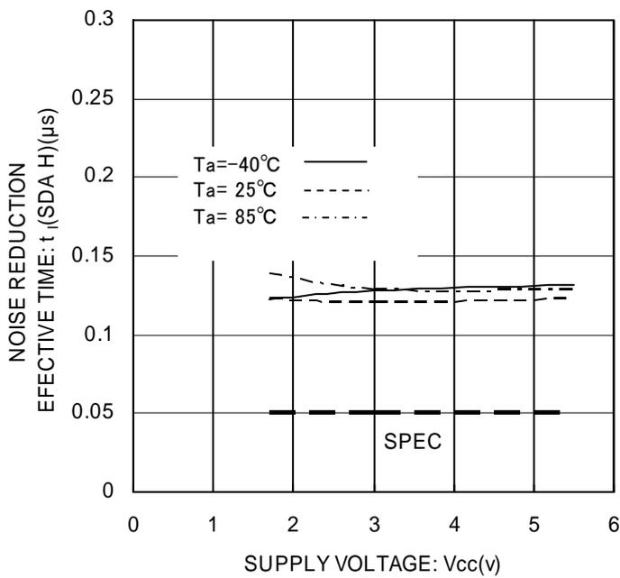
Figure 30. Noise Spike Width  $t_l$  (SDA H)
