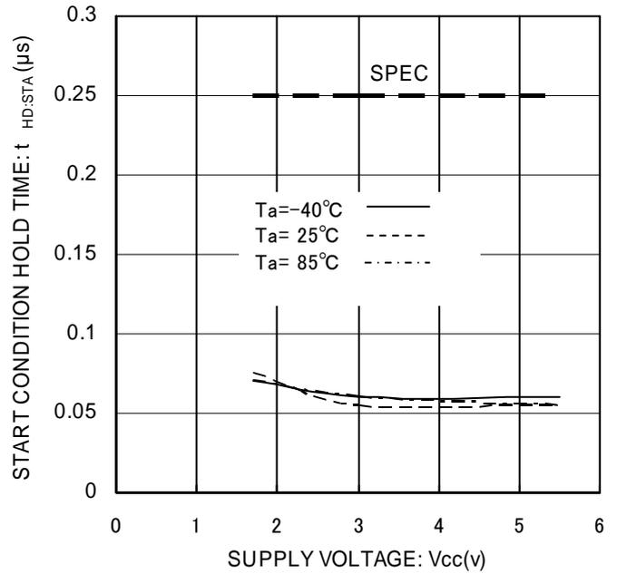
Figure 17. Start Condition Hold Time t<sub>HD:STA</sub>
