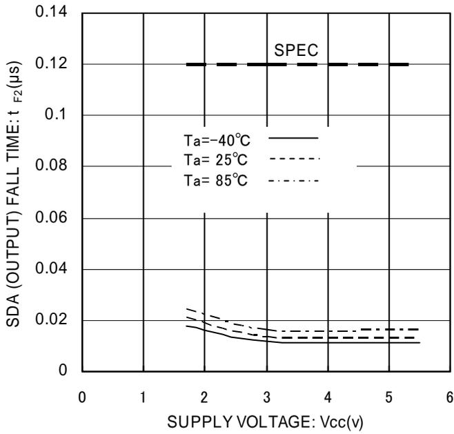
Figure 16. SDA (OUTPUT) Fall Time t<sub>F2</sub>
