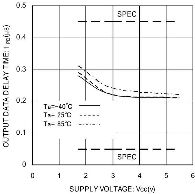
Figure 24. 'H' Output Data Delay Time tPD1
