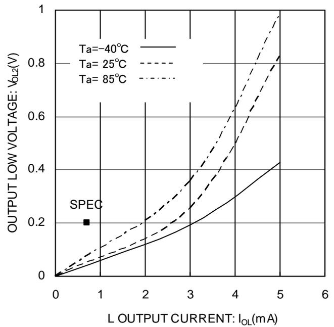
Figure 7. Output Low Voltage<sub>2</sub>  $V_{OL2}$  ( $V_{CC}=1.6V$ )
