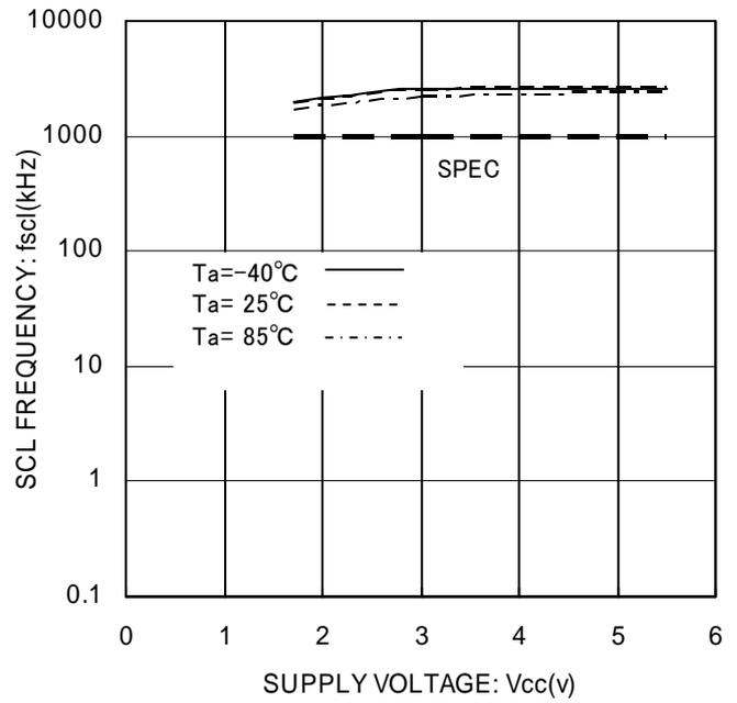
Figure 13. Clock Frequency f<sub>SCL</sub>
