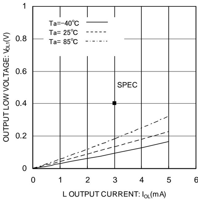
Figure 6. Output Low Voltage<sub>1</sub>  $V_{OL1}$  ( $V_{CC}=2.5V$ )
