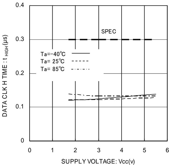
Figure 14. Data Clock High Period t<sub>HIGH</sub>
