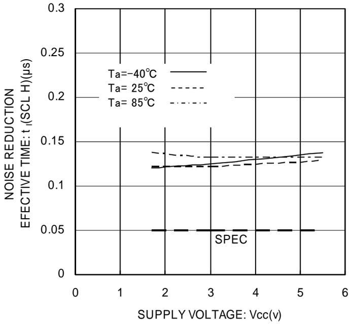
Figure 28. Noise Spike Width  $t_l$  (SCL H)
