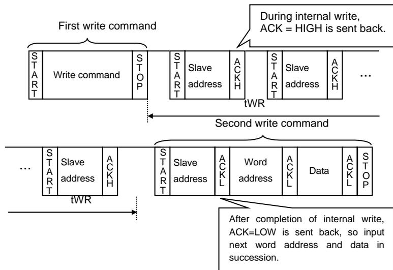
Figure 42. Case to continuously write by acknowledge polling
