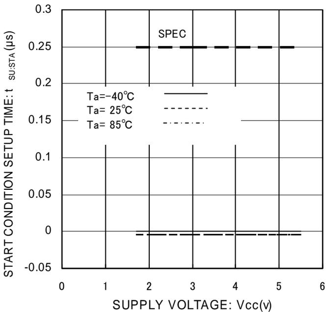
Figure 18. Start Condition Setup Time t<sub>SU:STA</sub>
