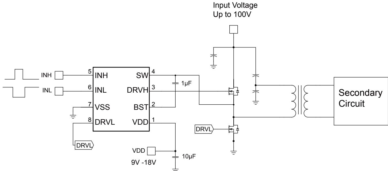
**Figure 4: Half-Bridge Converter**
