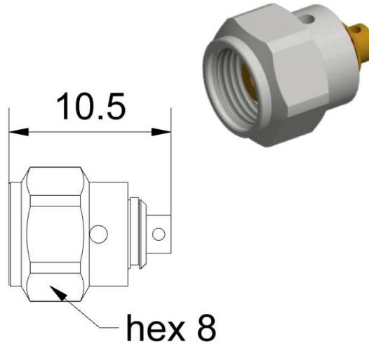
All dimensions are in mm; tolerances according to ISO 2768 m-H
