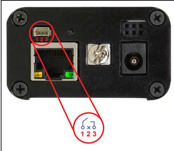
Figure 9. Relay terminal pin-out
