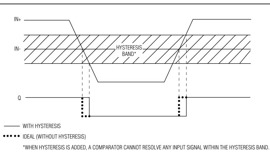
Figure 2. Effect of Hysteresis on Input Resolution
