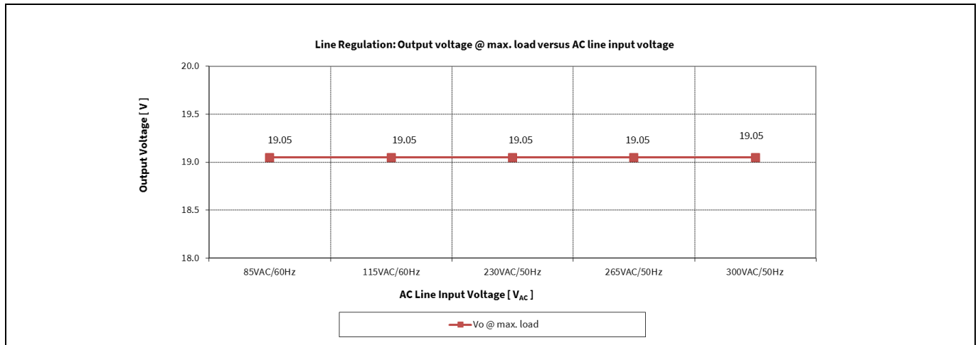
Figure 10 Line regulation V_{out} at full-load vs AC-line input voltage
