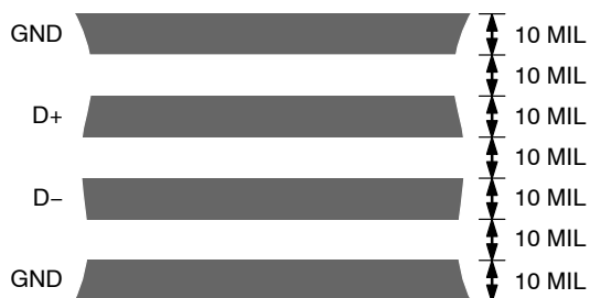
Figure 18. Typical Arrangement of Signal Tracks
