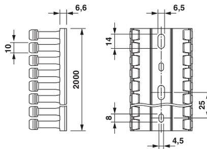
Base perforation according to DIN EN 50085
