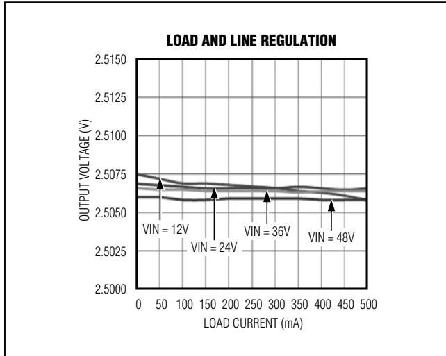
Figure 1. MAX17501H Load and Line Regulation
