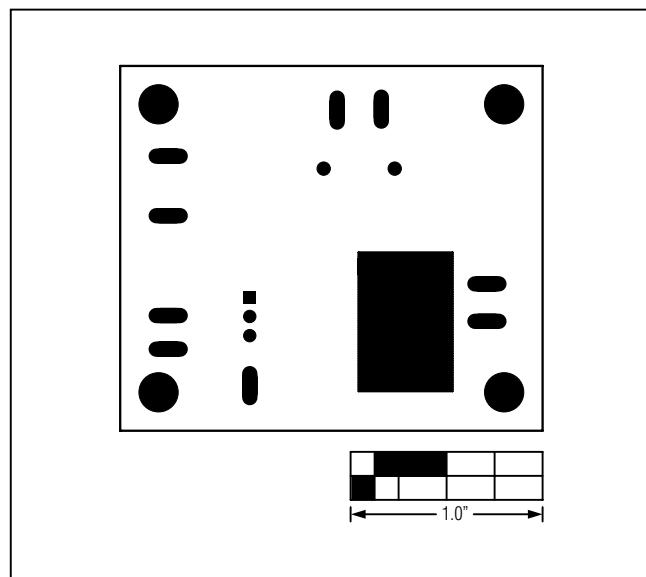
Figure 11. MAX17501H EV Kit PCB Layout—Bottom Solder Mask
