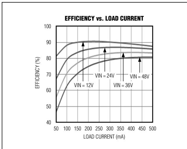
Figure 2. MAX17501H Efficiency
