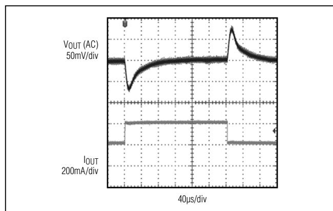
Figure 5. MAX17501H 250mA to 500mA Load Transient
