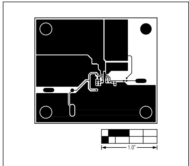
Figure 8. MAX17501H EV Kit PCB Layout—Component Side
