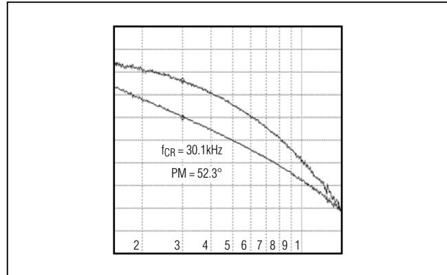
Figure 3. MAX17501H Full-Load Bode Plot
