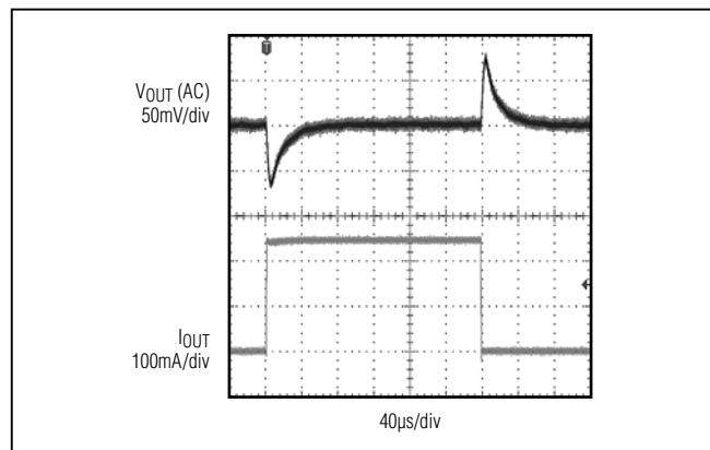
Figure 4. MAX17501H No Load to 250mA Load Transient
