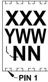
8-Lead DFN (2x3x0.9 mm)
