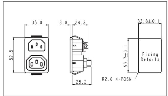
**SNAP FIT TO PANEL FUSED INLET/OUTLET**
