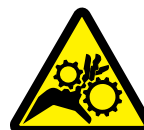
W3156 Gear Entanglement Hazard
