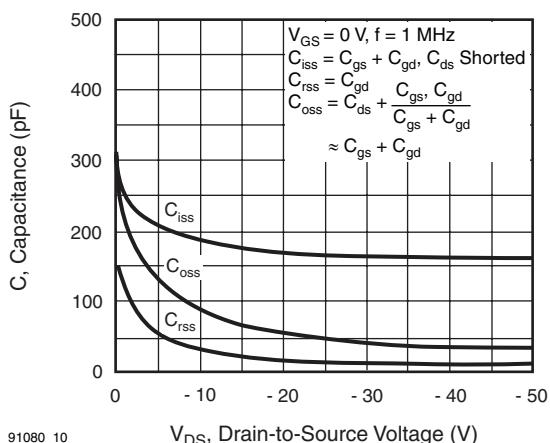
Fig. 10 - Typical Capacitance vs. Drain-to-Source Voltage
