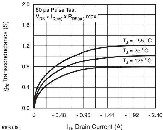
Fig. 6 - Typical Transconductance vs. Drain Current
