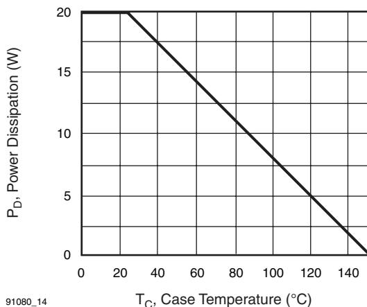
**Fig. 14 - Power vs. Temperature Derating Curve**
