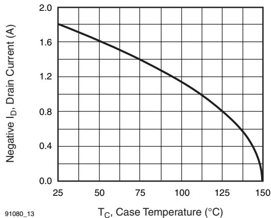
**Fig. 13 - Maximum Drain Current vs. Case Temperature**
