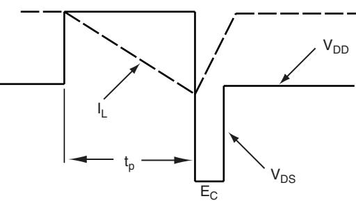
**Fig. 16 - Clamped Inductive Waveforms**
