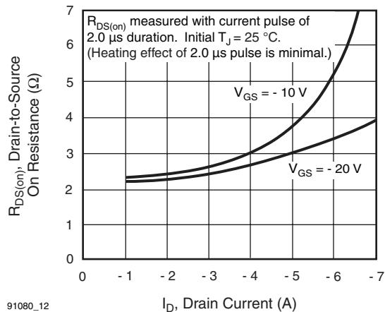
**Fig. 12 - Typical On-Resistance vs. Drain Current**
