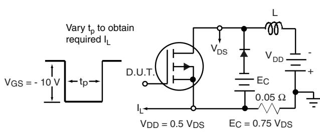
**Fig. 15 - Clamped Inductive Test Circuit**
