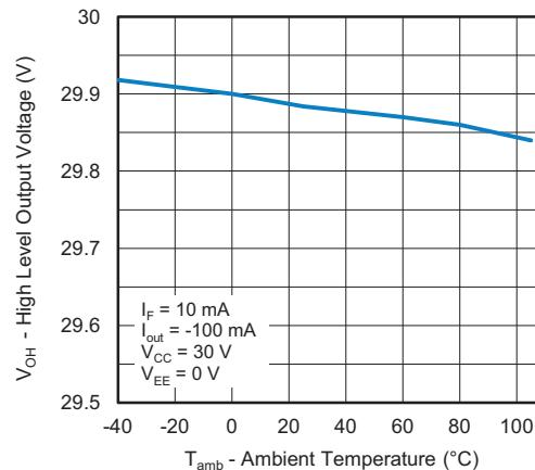
Fig. 8 - High Level Output Voltage vs. Ambient Temperature
