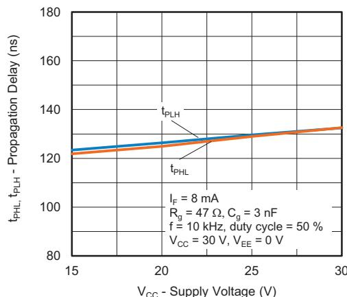
Fig. 14 - Propagation Delay vs. Supply Voltage
