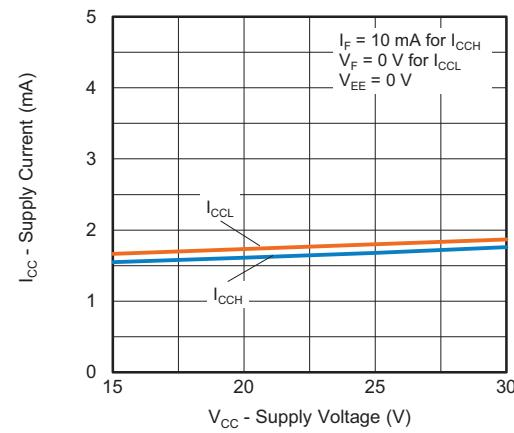
Fig. 17 - Supply Current vs. Supply Voltage
