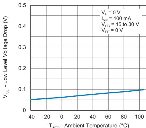
Fig. 11 - Low Level Voltage Drop vs. Ambient Temperature
