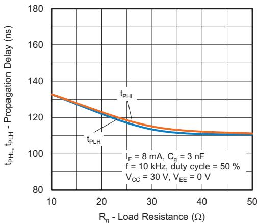
Fig. 15 - Propagation Delay vs. Load Resistance
