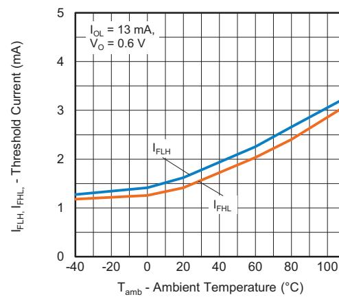
Fig. 7 - Threshold Current vs. Ambient Temperature
