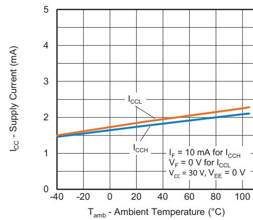
Fig. 18 - Supply Current vs. Ambient Temperature
