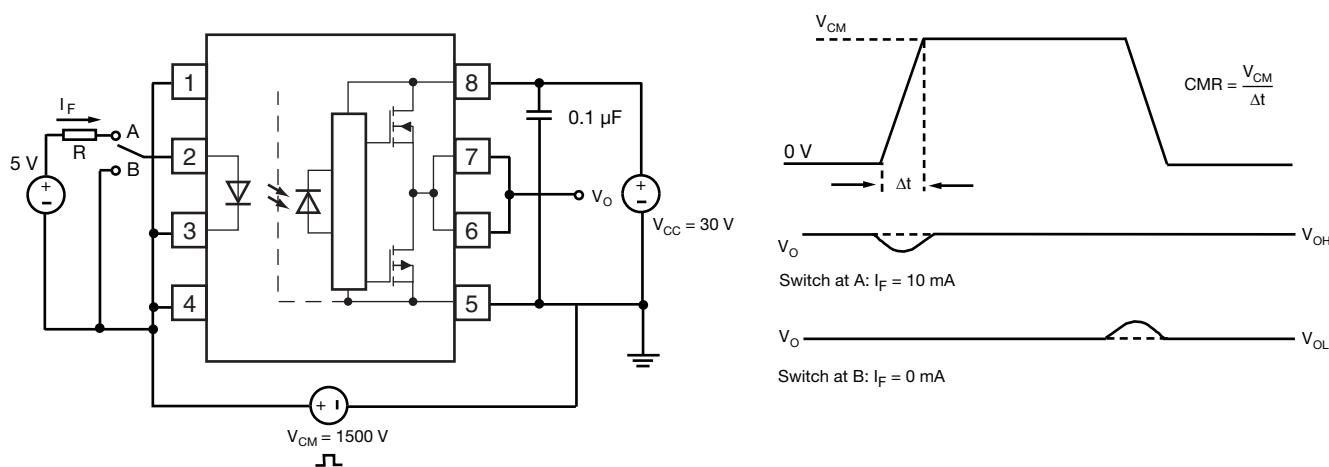
Fig. 4 - CMR Test Circuit and Waveforms
