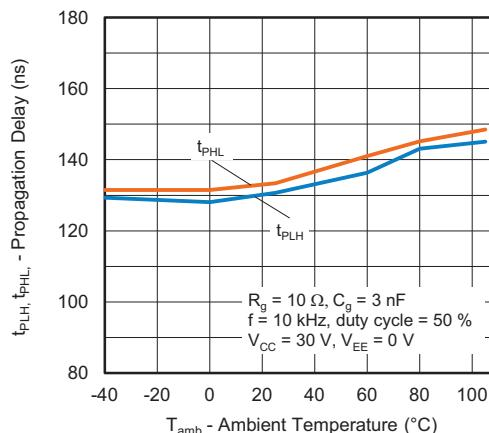
Fig. 13 - Propagation Delay vs. Ambient Temperature
