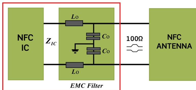
The matching circuit should be designed to match the IC impedance  $Z_{IC}$  to  $100\Omega$  and then connect the antenna through a  $100\Omega$  differential pair.
