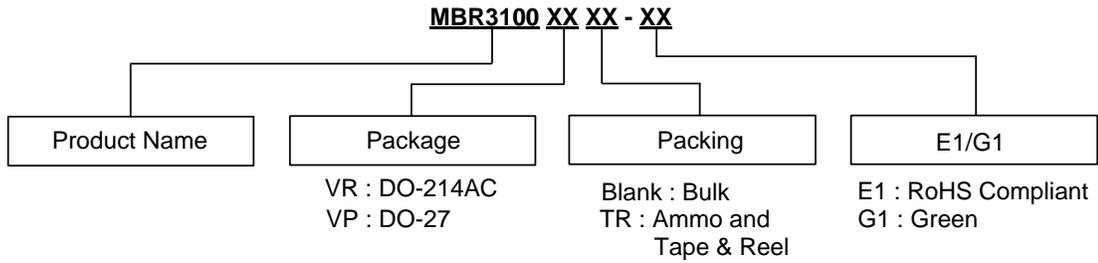
Note 4: Diodes Inc's Pb-free products, as designated with "E1" suffix in the part number, are RoHS compliant. Products with "G1" suffix are available in green packages.
