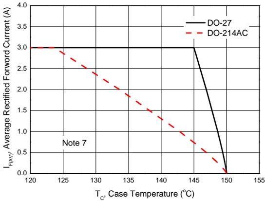
Figure 3. Average Rectified Forward Current vs. Case Temperature
