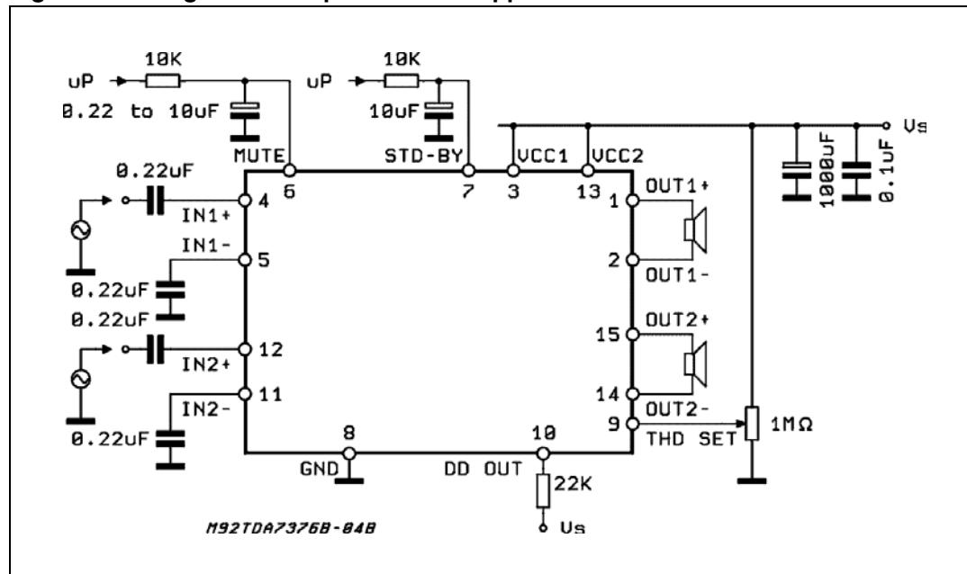
**Figure 17. Application board reference circuit**
