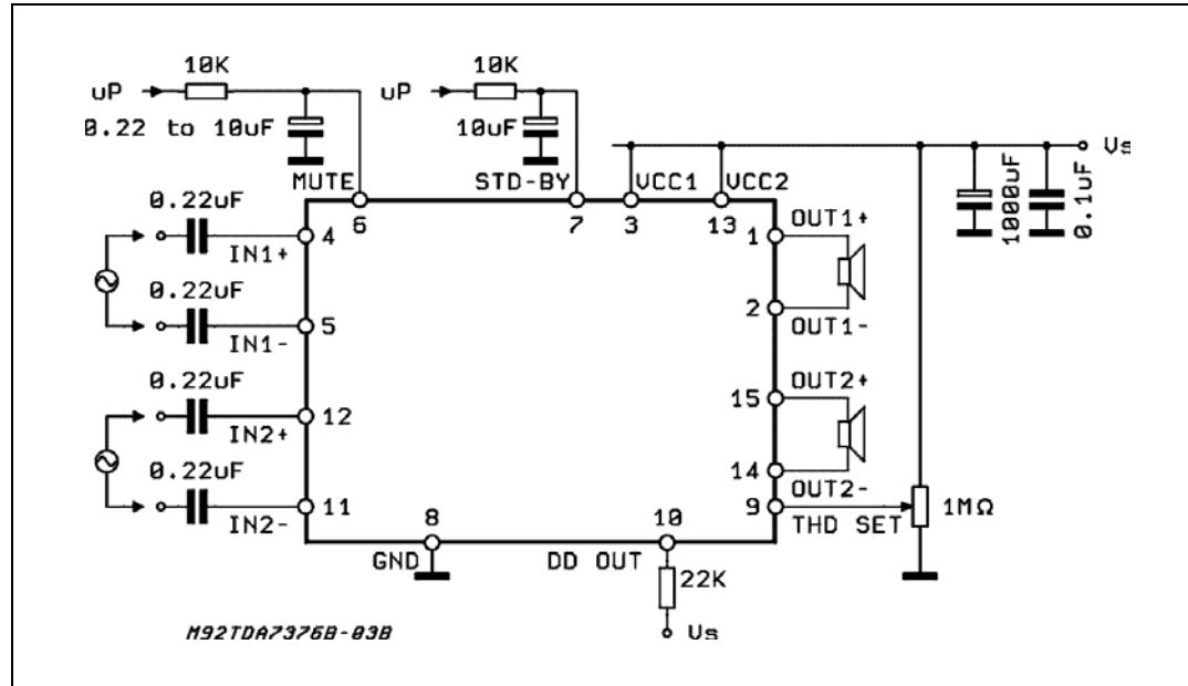
**Figure 16.** Single ended inputs test and application circuit
